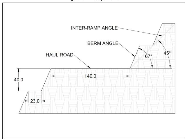
Figure 16-2: Pit Slope Profile
