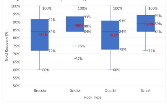
Figure 13-3: Gold Recovery and Rock Type Whisker Plot 1994 Bottle Roll Tests
