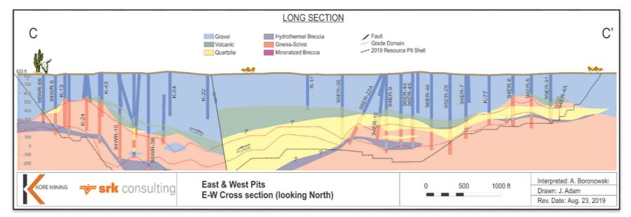
Figure 7-2: Conceptual East-West Long Section Across the Imperial Gold Deposit (looking North)
