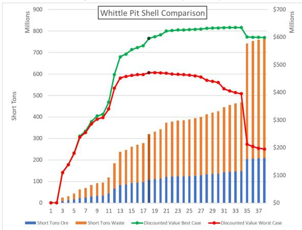
Figure 16-3: Whittle Pit Shell Comparison Graph
