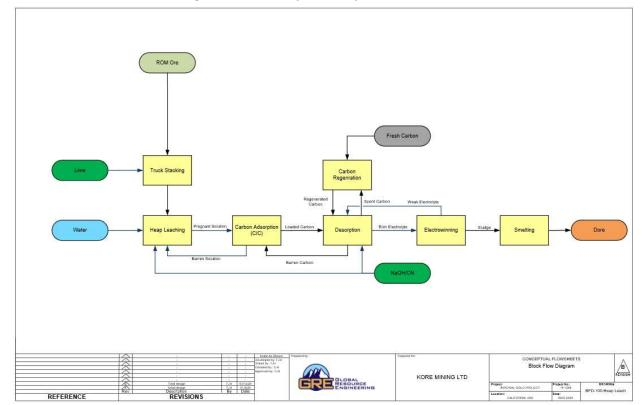
Figure 17-1: Conceptual Heap Leach Flowsheet
