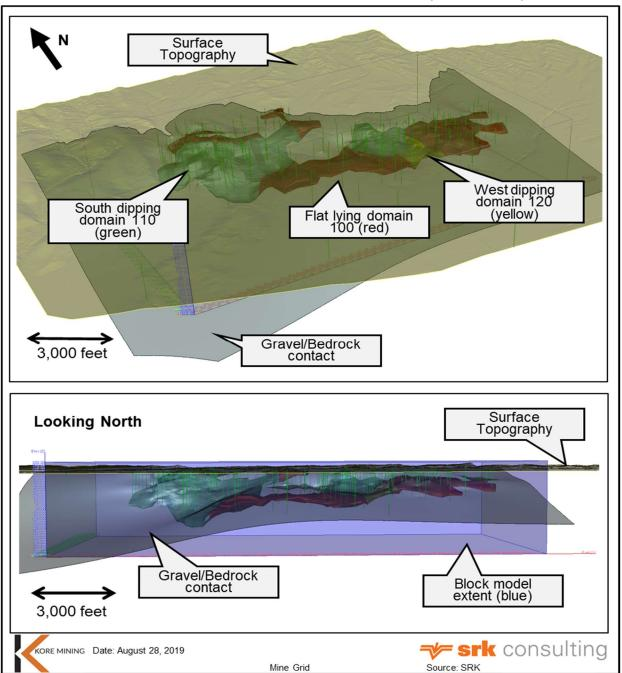
Figure 14-2: Cross-section Showing the Lithology-Gold Mineralization Relationship at the Imperial Gold Project
