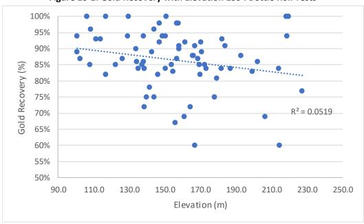
Figure 13-1: Gold Recovery with Elevation 1994 Bottle Roll Tests
