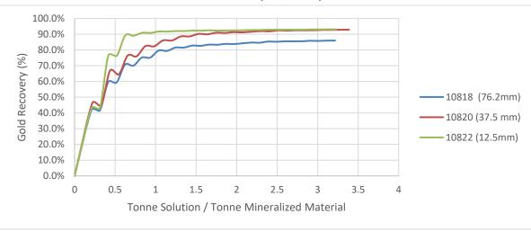
Figure 13-9: Final Gold Extraction Against Tonnes of Leaching Solution per Tonne of Mineralized Material (KCA, 1989)
