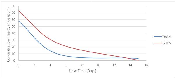
Figure 13-13: Cyanide Washing Profiles with Respect to Rinse Time for Tests 4 and 5 (Hazen Research, 1997)
