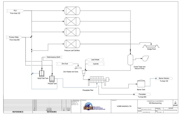
Figure 17-2: Merrill-Crowe System Schematic
