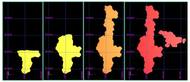
Within the phases, pits were designed with an overall pit slope of 45°, using a batter angle of 80°, bench height of 20 feet (doubled 10 feet benches). Catch berms are 16 feet wide. All in-pit haul roads were designed with a maximum 10% grade and a width of 90 feet (Figure 16-4).
