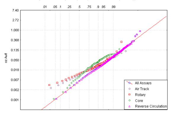
Figure 10-2: Long Valley Sample Distribution by Drill Type
