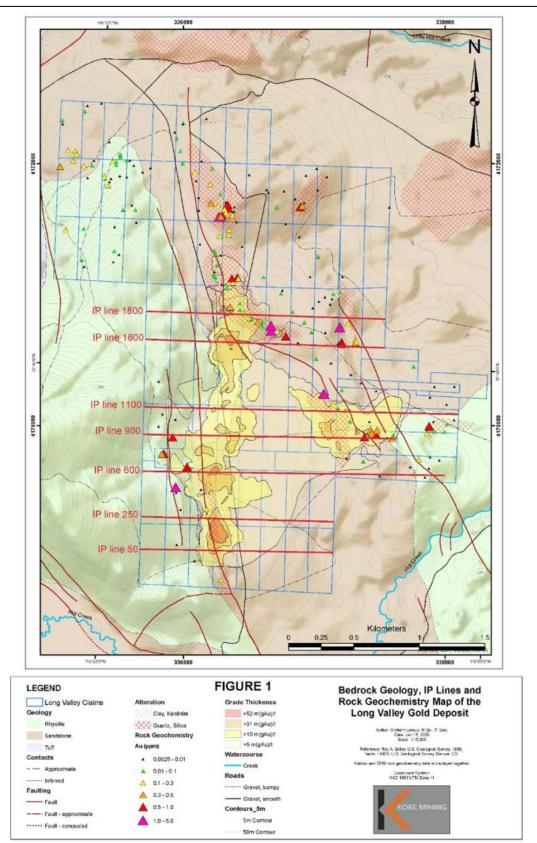
Figure 9-2: 2020 Surface Geology, IP Lines, Alteration and Grade-Thickness
