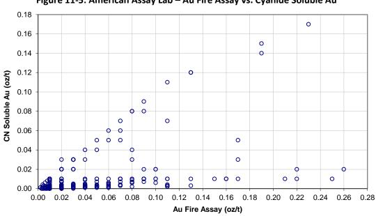
Figure 11-5: American Assay Lab – Au Fire Assay vs. Cyanide Soluble Au
