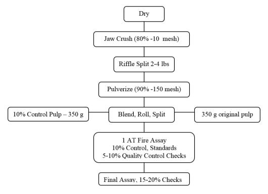
Figure 11-1: American Assay Lab Sample Preparation and Assaying Procedure
