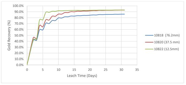
The final leaching solutions had a pH range of 9.7 - 10.2, and with concentrations between 0.15 g/L and 0.22 g/L. Cyanide consumptions ranged between 0.125 kg/t and 0.17 kg/t, and calcium hydroxide
