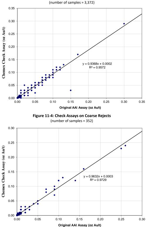
Figure 11-3: Check Assays on Sample Pulps
